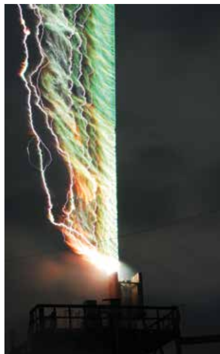
Figure 1: Triggered lightning from the tower launcher at the ICLRT. The copper triggering wire explodes at the right (straight vertical green line) with the wind blowing its remains to the left. Several downward leader/upward return stroke sequences (tortuous white channels) follow at hundredths of a second intervals, also blown by the wind to the left in this time exposure. (Photo by Dustin Hill).
